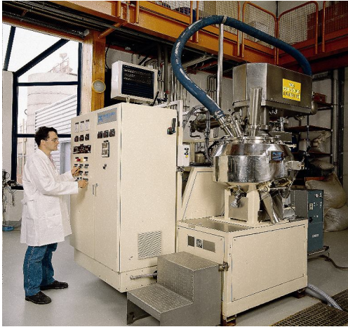
Figure 30: Batch and continuous microwave oven in industry
